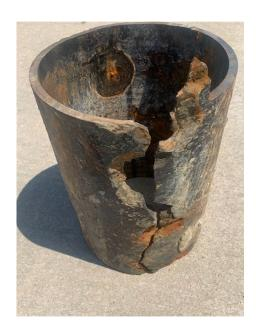
The Village has not taken on a major repair or replacement of pipes in the system for many years. There are sewer pipes in need of major rehabilitation and cast-iron water mains that are roughly 100 years old that need replacement. There were over 20 water main breaks from last fall to this winter. Pictured left is a piece of cast iron pipe from a recent Beverly Hills water main break.
